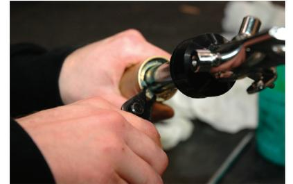
3. The lower fork leg should now pull apart (as shown at the left) We recommend wiping excess grease from the spring assembly to ease handling.
