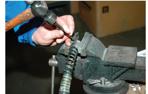
5. Clamp the aluminum spring retainer in a soft-jaw vice. Using an appropriate punch, unscrew the spring by striking the end of the spring wire. Once it has been loosened, it should unscrew by hand. Repeat procedure for the other end of the spring.
