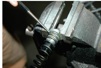
6. Screw the new springs onto the aluminum spring retainer by hand. Be certain that they are fully screwed on. Reassemble this fork leg and repeat procedure for the other fork leg.
