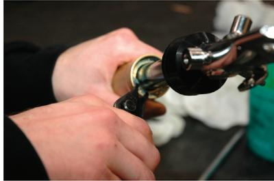
3. The lower fork leg should now pull apart (as shown at the left) We recommend wiping excess grease from the spring assembly to ease handling.
