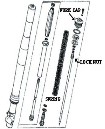
Check to make sure your oil level is 95mm. Please see your owners manual for instructions on doing this. Tighten the fork cap onto the lock nut to 14 lbf-ft. Thread the fork cap into the fork tube and torque to 25lbf-ft. Reset the rebound adjuster screw position and reinstall the forks. Torque the fork tube pinch bolts to 16lbf-ft.
