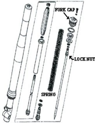
Check to make sure your oil level is 95mm. Please see your owners manual for instructions on doing this. Tighten the fork cap onto the lock nut to 14 lbf-ft. Thread the fork cap into the fork tube and torque to 25lbf-ft. Reset the rebound adjuster screw position and reinstall the forks. Torque the fork tube pinch bolts to 16lbf-ft.
