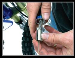
27. Install the slide into the carb and thread on the carb top. Be careful not to cross thread the carb top. It should thread on easily and smoothly.
