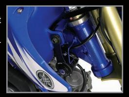
2. Remove the seat/rear fender/side panels by removing the (2) ten millimeter bolts under the rear fender.
