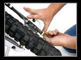
13. Install the BBR top triple clamp. Position the clamps as desired and tighten the lower perch bolts. Align the number plate bracket while assembling. Install and tighten the top nut and bolts.
