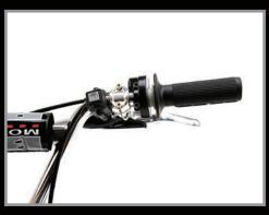
17. Install the brake lever on the right side of the handlebars. Install the start button also.
