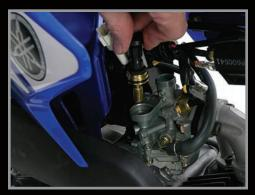
12. Cut the zip-tie holding the cables and wires to the frame, and you should now be able to remove the entire handlebar assembly.
