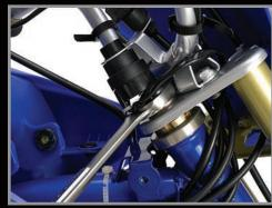
15. Insert the BBR choke into the carb. Be certain that the o-ring does not roll off during installation. Reinstall the choke clamp and phillips screw.
