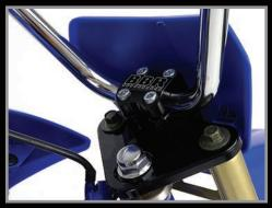
11. Use a 27mm wrench to remove the steering stem lock nut. If you remove the plastic lock nut that holds on the ignition key switch, it will give you enough room to remove the nut without removing the handlebars.
