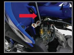
19. Install your key switch into the supplied bracket. Put the washer and nut on and tighten.
