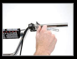
5. Disconnect the gray and white plugs just above the carb. The gray connector is for the kill switch. The white connector is for the starter button.
