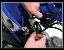
20. The key switch bracket mounts to the front coil screw. Remove the 8mm head screw and reinstall with the bracket.
