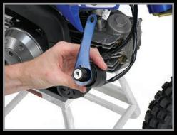
7. Unthread the carb top and pull it (along with the carb slide and spring) out of the carb.
