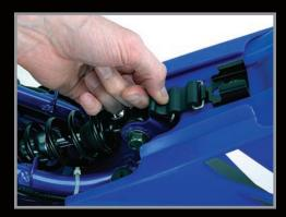
23. Reassemble the cable on the brake in the same manner as stock cable. Adjust brake as desired.
