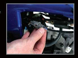
18. Route the wires for the kill switch and the starter button and connect them to the appropriate connectors. (They are color coordinated).
