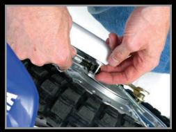
3. Turn off the gas using the fuel pet-cock on the left side of the motorcycle. Remove the rear gas tank strap and the two front tank bolts.
