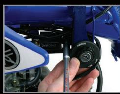
8. Pull back the spring and then unhook the carb cable from the carb slide. Retain the spring, slide, and needle for use with the BBR cable and carb top.
