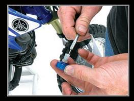
26. Install the cable onto the slide with the spring.
