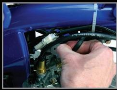
6. Using a long phillipshead screwdriver (arrow), remove the screw and retaining plate that holds in the choke. Pull out the choke cable and mechanism.
