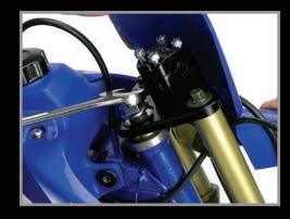
10. Remove the (2) 14mm head bolts at the top of the fork legs. If you do not support the front wheel, it can drop down once these bolts are removed.
