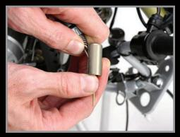
9. Remove the front brake cable by unthreading the adjuster at the bottom of the front brake mechanism. Use a 12mm wrench to remove the cable lock nuts from the fork.
