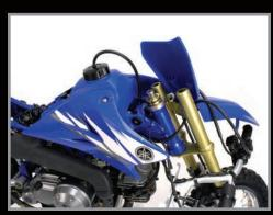
16. Install the kill switch on the left side handlebar.
