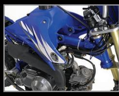
24. Install the cable into the throttle and install the throttle on the handlebars. At this point you can glue the grips on. Be careful not to get glue under the throttle and restrict throttle movement.
