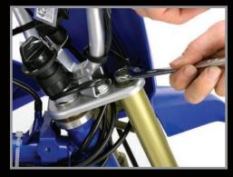
14. Install the handlebars In the clamps, position, and tighten with the 6mm allen wrench.
