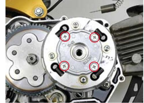
15. Straighten the tab of the clutch lock nut lock washer. Remove the clutch lock nut with the appropriate special clutch tool. It is available from Honda as part #07716-0020100.
