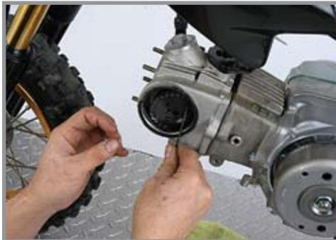
42. Once the sprocket has been installed, double check that the flywheel is on the "T" mark and the notch on the cylinder head is pointing at the "O" on the sprocket. Torque bolts to 6.5 ft.lbs. Rotate the flywheel slowly by hand and check for any interference.
