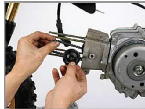
9. Remove the cylinder from the engine cases. The base gasket may also be difficult to release. Again, a rubber hammer can be used with care.
