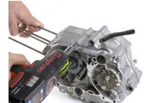
31. Install the kickstart shaft with spring into the right side of the motor.
