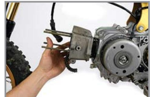
38. Feed the timing chain up through the cylinder and install the 6mm bolt (10mm head) to retain the cylinder to the engine cases. Slide the timing chain roller into the cylinder and install its bolt.
