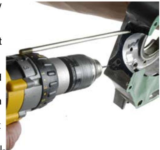
30. Install the 7 bolts that hold the crankcase halves together. Tighten in a crisscross pattern.
