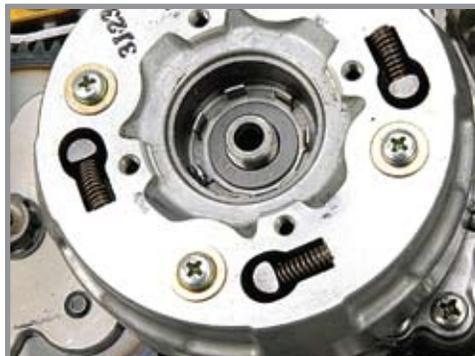
50. Install the clutch lifter cam plate, the "oil-through-spring" and "oil-through-tube". Next install the spring, ball retainer, and the clutch lifter arm. Finally, reinstall the clutch cover (right side engine case), kick-starter and brake pedal.
