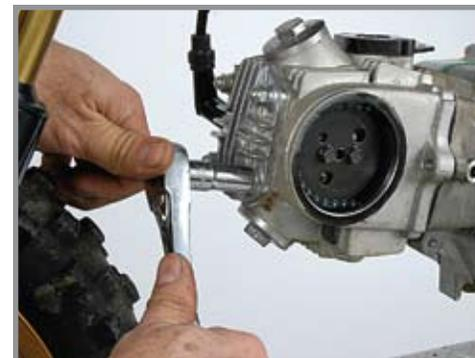
6. Remove the camshaft sprocket from inside the left of the cylinder head by removing its (2) 6mm bolts (8mm heads).
