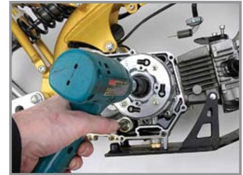
16. Remove the oil pump by removing the (3) Phillips head screws.
