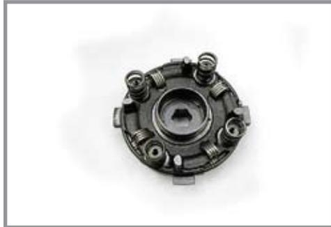
48. Once the clutch is assembled, you can insert the clutch buffer springs from the front side. Insert the back of the spring into the cast iron inner basket. Use a screwdriver to compress the spring and slip it into the out basket's tang.
