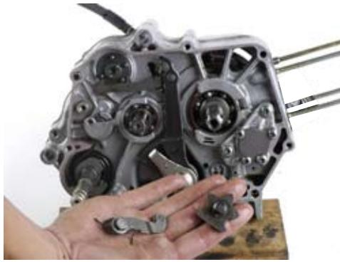
33. Install cam chain and ignition stator base.
