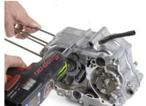
25. Place the engine left side down on supports (old 2 X 4's work well). Separate the right and left crankcase halves. May help to tap transmission shaft and crankshaft with rubber hammer.
