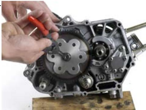
20. Remove primary gear, bushing and spacer. These parts will need to be installed on your new crank.
