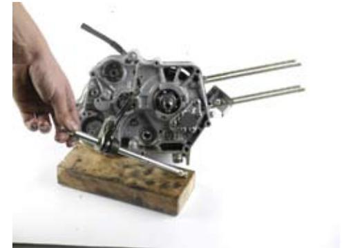
24. Loosen and remove the crankcase bolts (7).
