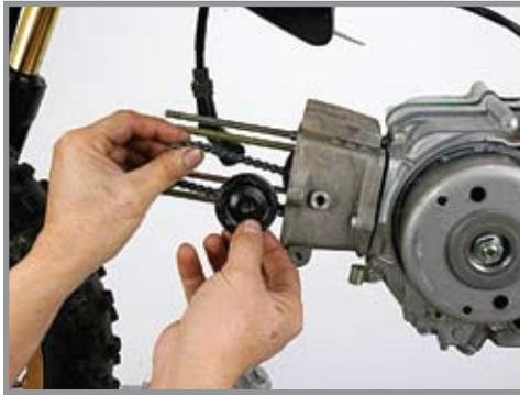
39. Slide the head gasket onto the head studs and install the o-ring. A small amount of grease on the o-ring can help hold it in place. Then slide the cylinder head onto the head studs. Feed the timing chain up through the cylinder head.
