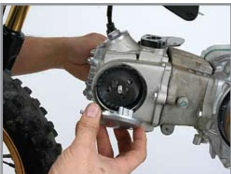
4. Remove the (3) 6mm bolts (10mm heads) that hold the timing chain roller (shown) and the cylinder head to the cylinder and the cylinder to the engine cases.
