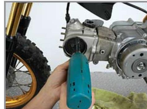
7. Remove the cylinder head, gasket, and 2 dowels. Some force may be required to release the head gasket. A rubber hammer may be useful. Be careful not to damage the cylinder or cylinder head. DO NOT use a screwdriver to pry the components apart or damage will occur.
