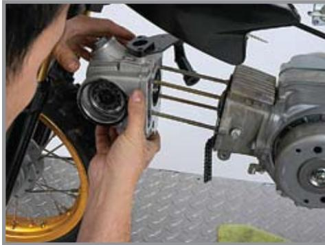
40. When installing the top cylinder head cover make sure the arrow on the cover is pointing down. Place the copper washer onto the bottom left bolt. Place the plain nut onto the bottom right bolt.
