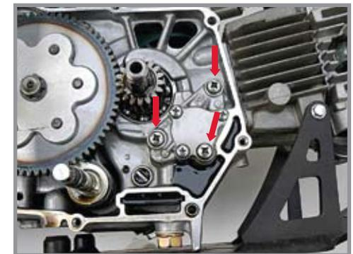
17. Remove ignition stator base (2 phillips head screws).
