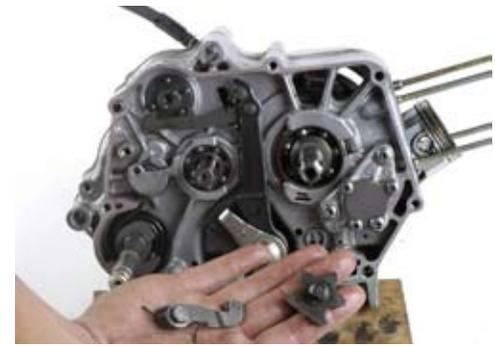
22. Remove the snap ring from the kickstarter shaft, disconnect the return spring, and slide off the retainer.
