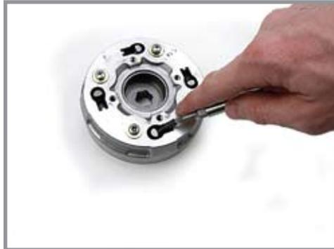
49. Reinstall the clutch assembly onto the crankshaft. Install the 14mm tabbed lock washer, then the conical lock washer (with the words "OUT SIDE" facing out), and then the lock nut. Use the special clutch tool to torque the nut to 12-15ft. lbs.
