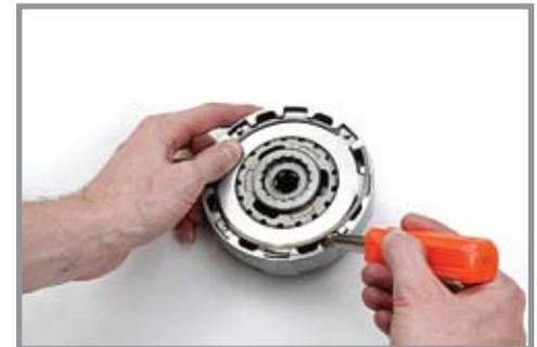
46. Remove the (4) Phillips head screws on the front of the clutch basket.
