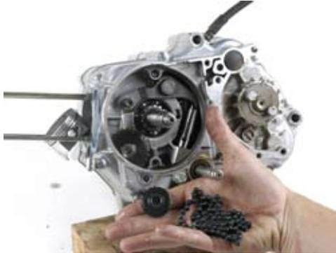
19. Remove the snap ring retaining the driven gear and remove gear.
