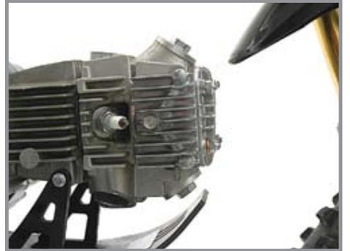
52. Using a 9mm wrench, loosen the lock nut and rotate the adjuster until your feeler gauge measures as follows:
