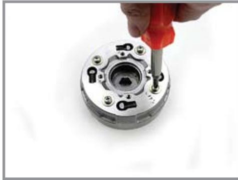
47. Pull the outside of the basket off exposing the clutch springs. Note that the (4) small buffer springs will fall out. Replace the clutch springs with the BBR HD clutch springs. Reassemble the clutch.
