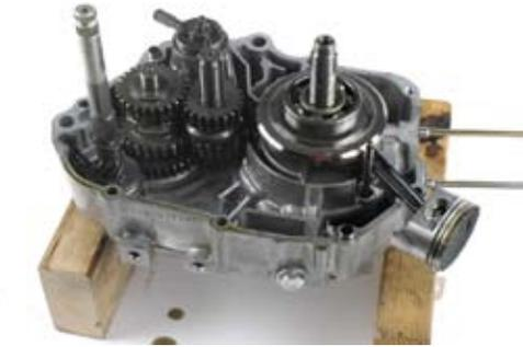
27. Clean the crankcase mating surfaces before assembling.
