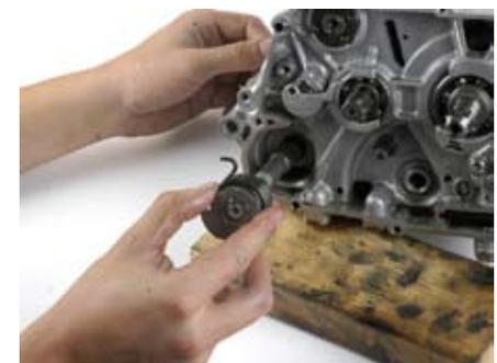
32. Install the bolt and washer on the shift drum. Install drive gear. Install primary gear, bushing and spacer removed from OEM crank.
