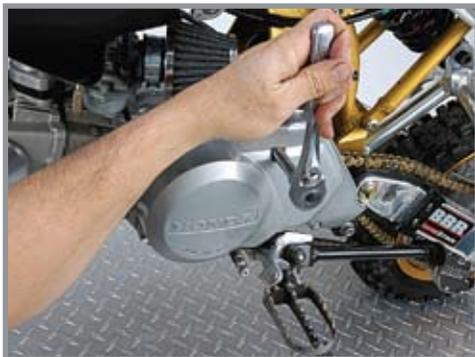
Remove countershaft sprocket.
