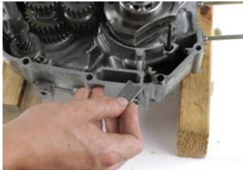
28. Install BBR crank into left crankcase.
