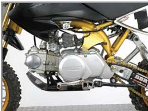
2. Remove the left side cover (flywheel cover) by removing the (3) 6mm bolts (8mm heads).
