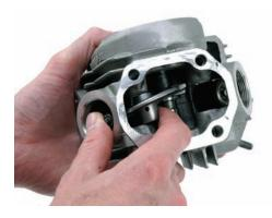
13. Remove one of the small piston clips from inside the piston (use a small screwdriver or needle-nose pliers). Push out the piston pin, and remove the piston from the rod. Use care not to drop the clip into the engine cases. Place a rag in the engine openings to prevent this.
