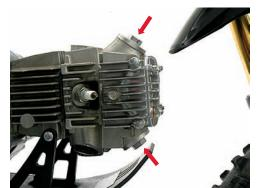
Fill with engine oil and check that everything is tight and in place. Oil capacity is .6 US qt. for a refill. A complete engine rebuild requires .8 US qt. of oil. Typical warm up procedures, as described in your owners manual, should be followed to allow for proper breakin.
