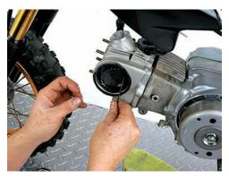
**25.** Set engine to Top Dead Center. Using a 9mm wrench, loosen the lock nut and rotate the adjuster until your feeler gauge measures as follows:
