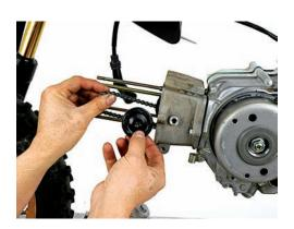
and remove the rocker arm shafts.
