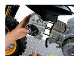
11. Remove the cam-chain roller from inside the cylinder by removing the 6mm bolt (10mm head). Needle nose pliers may be helpful to remove the roller from inside the cylinder.
