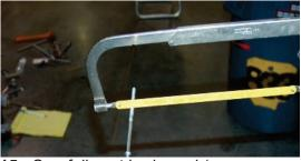
**15.** Carefully cut brake rod (we recommend using a hack saw) leaving 3/4" of threads then install the brake rod adapter as shown.
