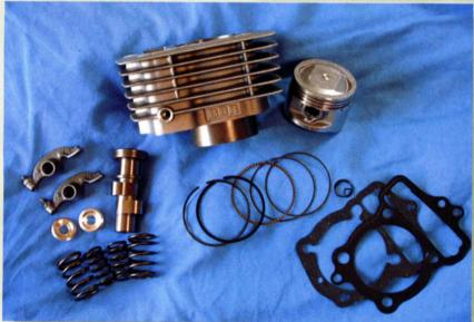
four-stroke without some of the complexity of the four-valve race engines or the shim-under-bucket designs that take much more mechanical skill than the simple screw-tappet design here. If you remove the studs when replacing the cylinder, the work can be done with the motor in the chassis, too. It takes about three hours to do the work if you have all the tools; replacing the valve springs is the trickiest
