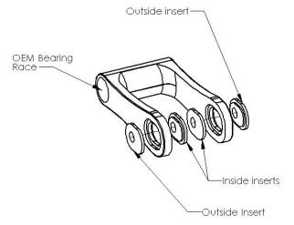
Align insert hole with swingarm linkage. This is easiest accomplished by raising or lowering the swingarm and the BBR linkage until they line up. When holes are aligned install outside insert and bolt through BBR linkage and swigrm linkage. Install other outside insert and nut .
