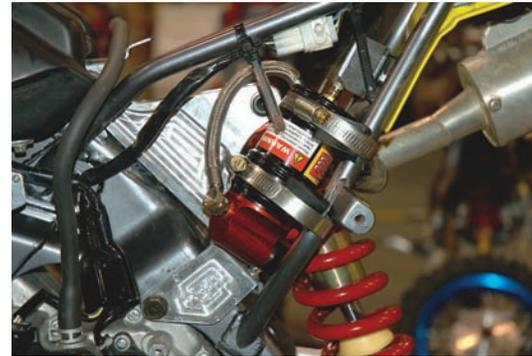
10. Install shock with reservoir hose pointing towards the rear fender.
