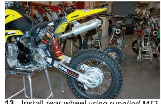
13. Install rear wheel using supplied M12 Fuji Locknut on OEM axle.
