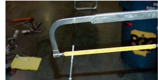
15. Carefully cut brake rod (we recommend using a hack saw) leaving 3/4" of threads then install the brake rod adapter as shown.
