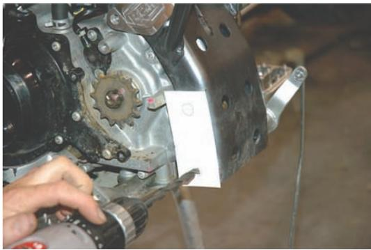
6. Drill frame for chain roller using the provided template to locate the hole.
