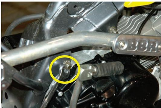
8. Remove center engine bolt.
