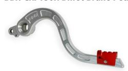
This lightweight billet 6061 T-6 aluminum brake pedal replaces the stock steel pedal adding strength and saving weight. With three different tip location settings, it allows the rider to customize the fit and function of this important control. Pre-drilled for a brake snake, this brake pedal is ready to race, just bolt it on.
