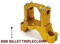
Designed to accommodate adult riders. Raises bar mount position 11/4", fully adjustable forward and backward. Allows lowering of forks by 1" to raise front end or retain stock height. Perfect match for BBR swingarm.
